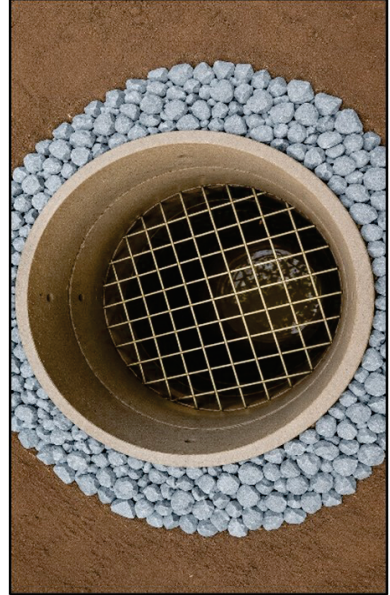
Figure 5.4. Percolation Pit. Source: Created by the authors using AI-assisted illustration (2026).
