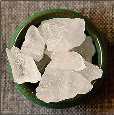
Figure 4.3. Alum Treatment for coagulation and clarification of harvested rainwater. Source: Authors photograph
