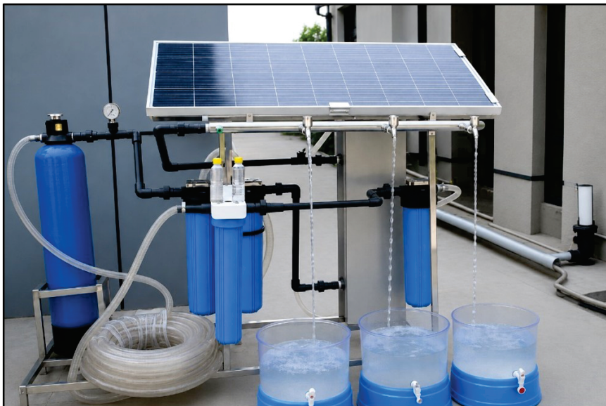
Figure 4.5. Solar Water Purifier (SWP) for treatment of harvested rainwater using solar energy. Source: Created by the authors using AI-assisted illustration (2026).
